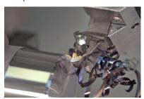
$v_c = 160 \text{ m/min}$ = 5.0 mm  $f = 0.35 \, \text{mm/U}$
